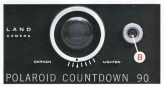
**B.** The electric eye: The electric eye only works for non-flash pictures. When you press No. 2 button, the shutter opens. Instantly, the electric eye measures the brightness of the light reflected from the subject and times the closing of the shutter to give correct exposure.
