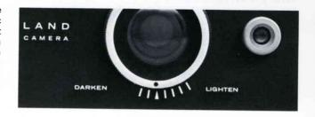
**D.** The flash Lighten/Darken control: Turning this L/D control adjusts the amount of light coming from the flash unit so you can make a flash picture lighter or darker than it would be if the L/D control were left at the Normal position (shown here). For more details about its use, see page 35. This control has no effect on pictures made without flash.
