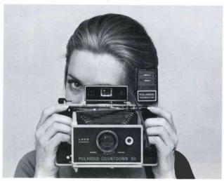
**HORIZONTAL:** Grip the two ends. Place your forefingers on the No. 1 buttons; you can easily shift the right forefinger to the No. 2 button. To steady the camera, press your elbows into your ribs; rest the camera against your nose.
